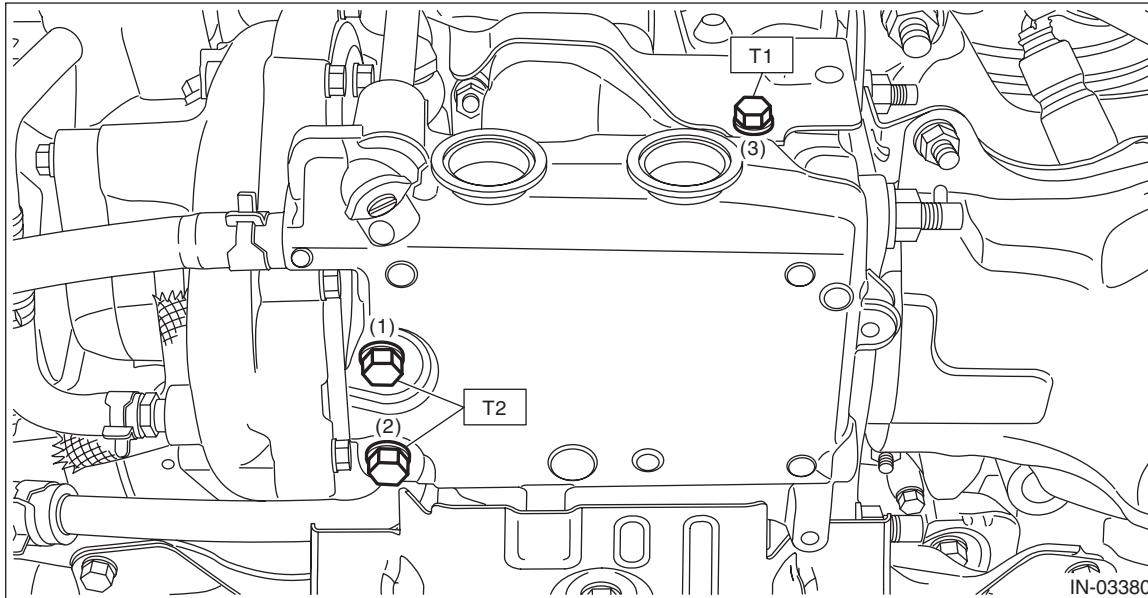
2) Connect the turbocharger hose to the oil pipe.
