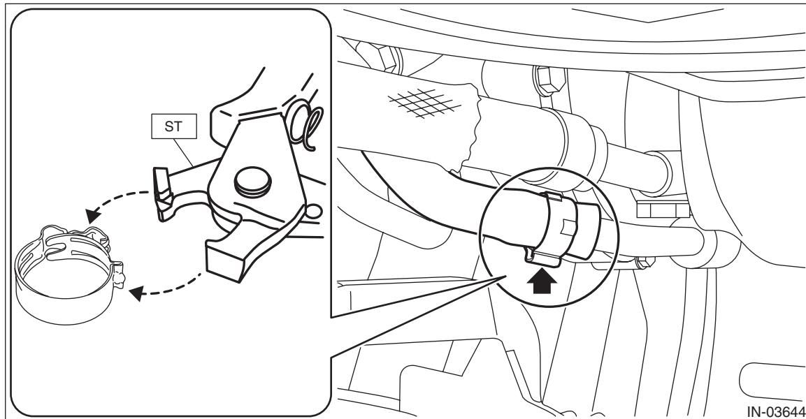
6) Install the air intake duct. <Ref. to IN(w/o STI)-22, INSTALLATION, Air Intake Duct.>
